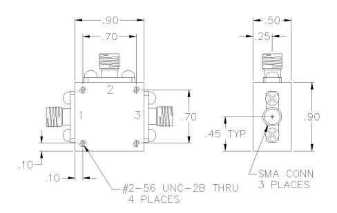
Name: C3-07-414 Frequency Range: 1-750 MHz Coupling:  $15.0 \pm 0.5 \, dB$ Coupling Flatness: ±0.40 dB max. Insertion Loss: 1.2 dB max. Directivity: 23 dB min. VSWR:
