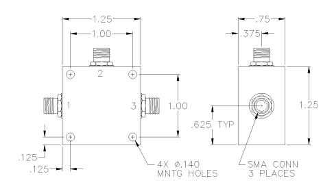
Name: C1-10-411 Frequency Range: 1-2000 MHz  $10.0 \pm 1.0 \text{ dB}$ Coupling:
