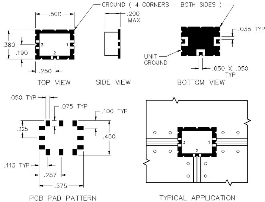
ALL NON-USED PORTS AND UNIT GROUND SHALL BE GROUNDED TO THE MAIN BOARD
